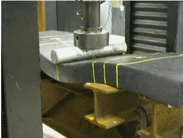
4300# load on 20" beam centers.
