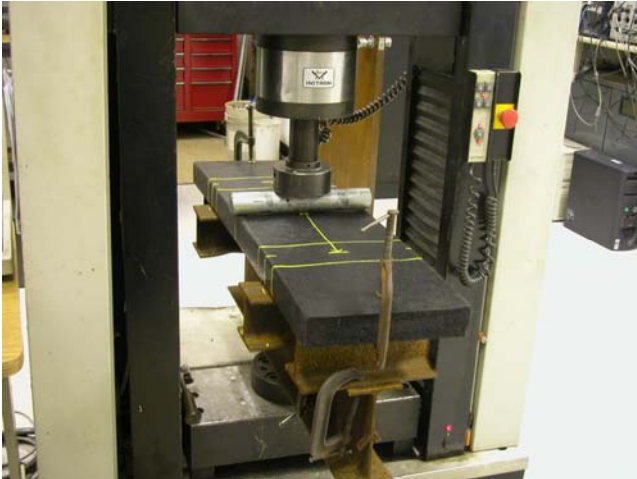
Point load application with 20" beam centers. 2" diameter bearing rod across width.
