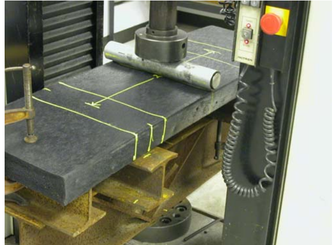
Point load application with 20" beam centers. 2" diameter bearing rod across width.
